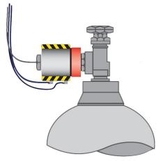
The Auto-Guard<sup>TM</sup> connection cover remains in the extended position when a manifold is online or any condition exists where it is unsafe for operators or equipment to open the cylinder connection fitting.
