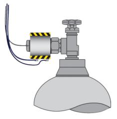
The Auto-Guard<sup>™</sup> Connection cover retracts into its housing, revealing the cylinder connection fitting for operator access after the controller determines the system conditions are safe. The Auto-Guard<sup>™</sup> will remain in this position until the cylinder change and leak test have successfully been completed.
