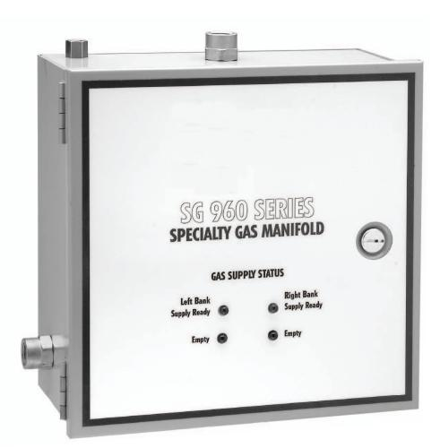
The SG960 fully automatic switchover manifold for high purity gases. An integrated circuit board monitors and displays cylinder bank pressure and delivery pressure electronically. Change-overs occur automatically eliminating the need to manually reset levers or valves.
